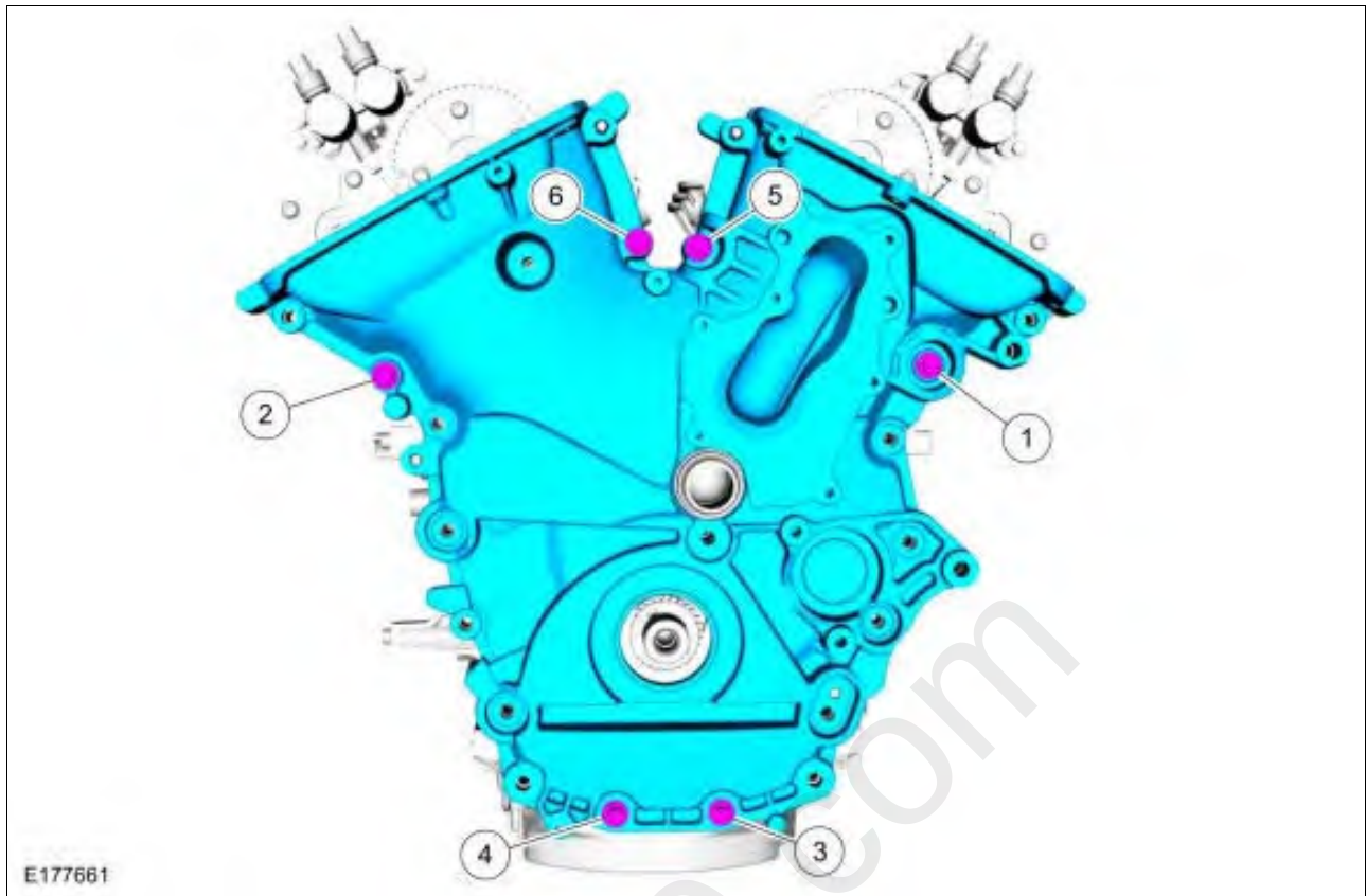
Fig 12: Engine Front Cover Bolts Tightening Sequence
